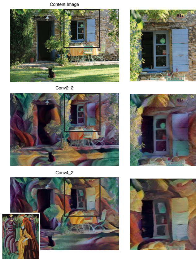
Figure 5. The effect of matching the content representation in different layers of the network. Matching the content on layer ‘conv2_2’ preserves much of the fine structure of the original photograph and the synthesised image looks as if the texture of the painting is simply blended over the photograph (middle). When matching the content on layer ‘conv4_2’ the texture of the painting and the content of the photograph merge together such that the content of the photograph is displayed in the style of the painting (bottom). Both images were generated with the same choice of parameters ( \alpha/\beta = 1 \times 10^{-3} ). The painting that served as the style image is shown in the bottom left corner and is named Jesuiten III by Lyonel Feininger, 1915.
